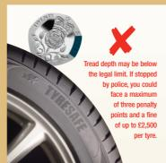
To check your tread, simply insert a 20p coin into your tyre's tread grooves and check whether the rim of the coin is covered by the tread. Do this check in the main tread grooves across the width of the tyre and repeat at several locations around its circumference. If you can see the rim of the coin the tyre tread may be worn close to the legal limit of 1.6mm and needs to be checked by a tyre specialist.
